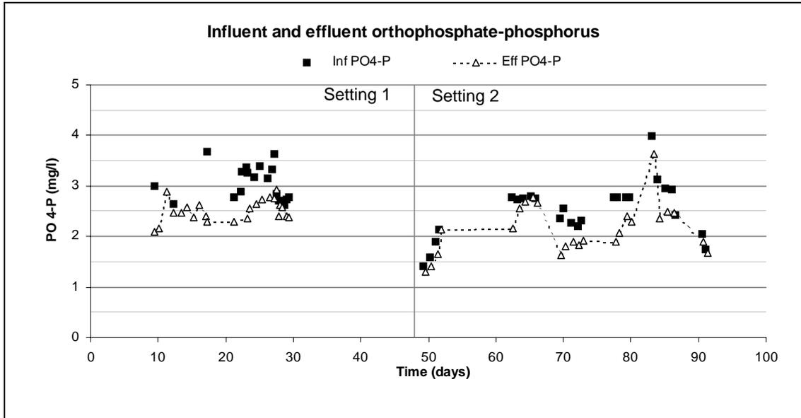
**Figure 4.3. Influent (Inf) and effluent (Eff) orthophosphate-phosphorus (PO<sub>4</sub>-P).**
