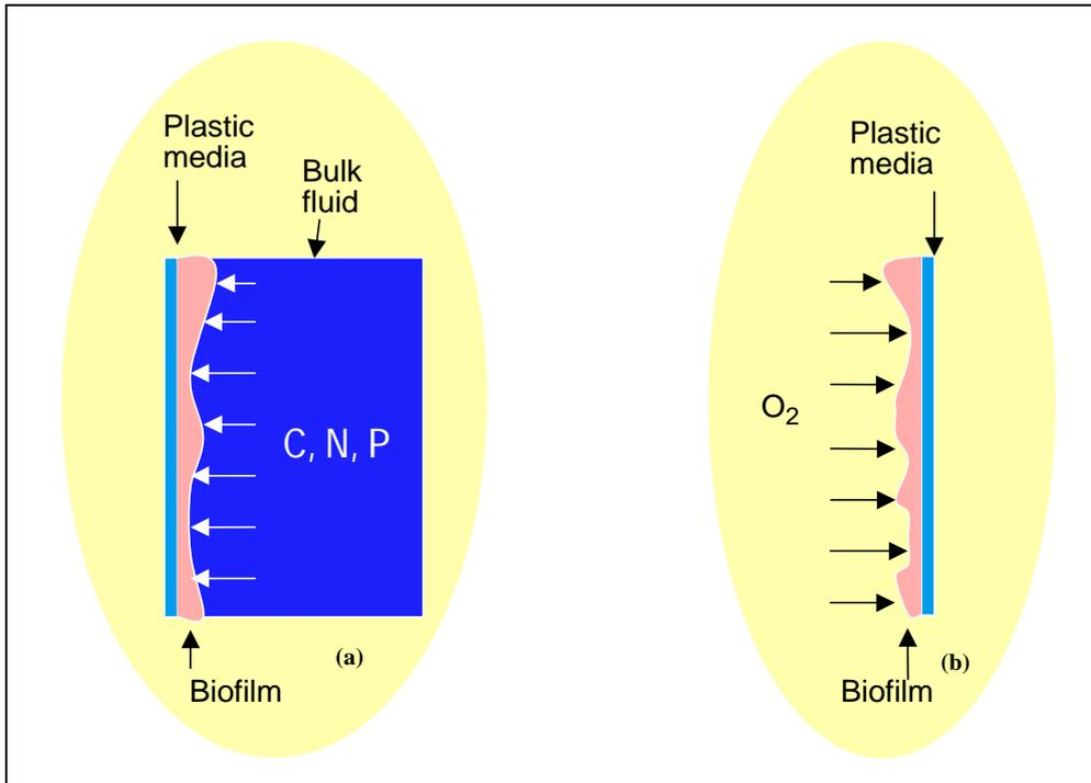
**Figure 3.7. (a) Biofilm submerged, and (b) biofilm exposed.**
