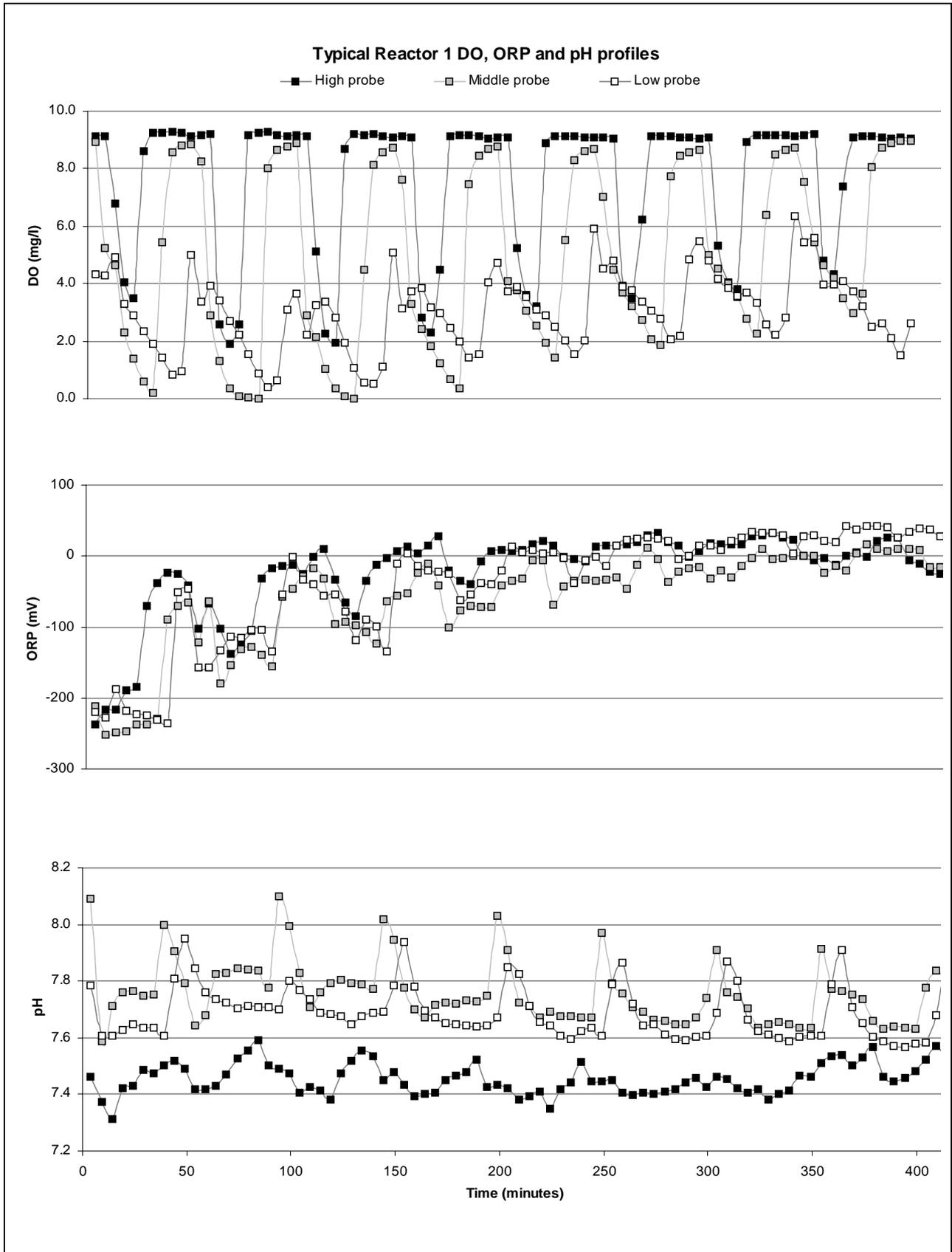
Figure 4.7. Typical Reactor 1 dissolved oxygen (DO), oxidation–reduction potential (ORP) and pH profiles for one treatment cycle.
