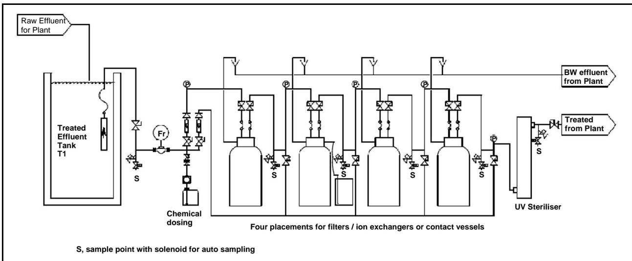
Figure 5.3. Overall schematic of the tertiary treatment system installed at the Water Research Facility.
