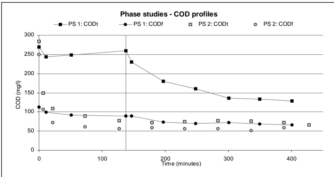
Figure 4.5. Chemical oxygen demand (COD) profiles for Phase-study (PS) 1 and 2 (vertical line represents the anaerobic phase for PS 1) (COD<sub>t</sub>, total COD; COD<sub>f</sub>, filtered COD).
