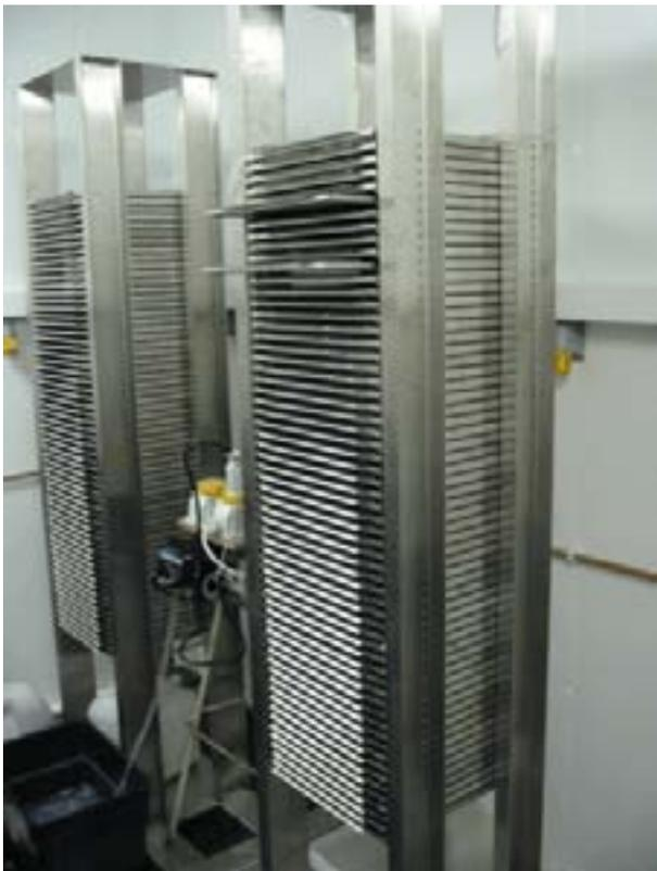
Figure 6.2. Laboratory horizontal flow biofilm reactor units.
