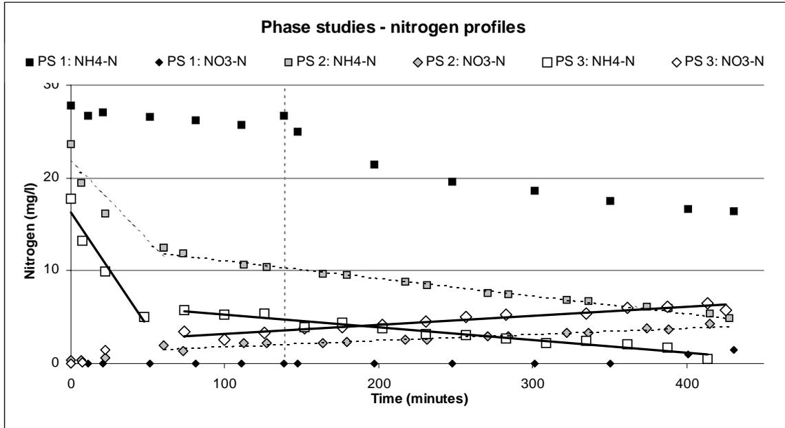
Figure 4.6. Phase study nitrogen profiles (vertical dashed line represents the anaerobic phase for Phase-study (PS) 1) (NH<sub>4</sub>-N, ammonium-nitrogen; NO<sub>3</sub>-N, nitrate-nitrogen).
