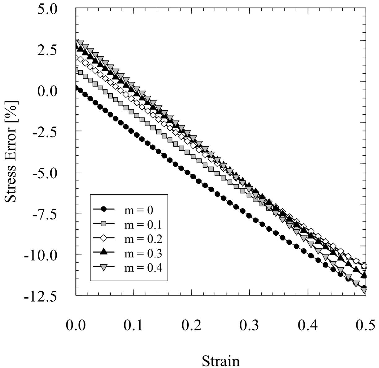
**Figure 11: Relative error in stress from isothermal models with combined friction effects and heating from plastic deformation ( $T=1100^{\circ}\text{C}$ ,  $\dot{\epsilon}=1\text{s}^{-1}$ ,  $\eta=0.9$ ).**
