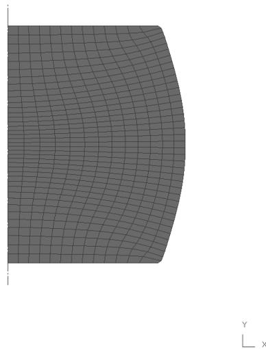
**Figure 4: Typical deformed mesh of isothermal compression test model ( $T=1100^{\circ}\text{C}$ ,  $\dot{\epsilon}=1\text{s}^{-1}$ ,  $\epsilon=0.5$ ,  $m=0.3$ , no re-meshing)**
