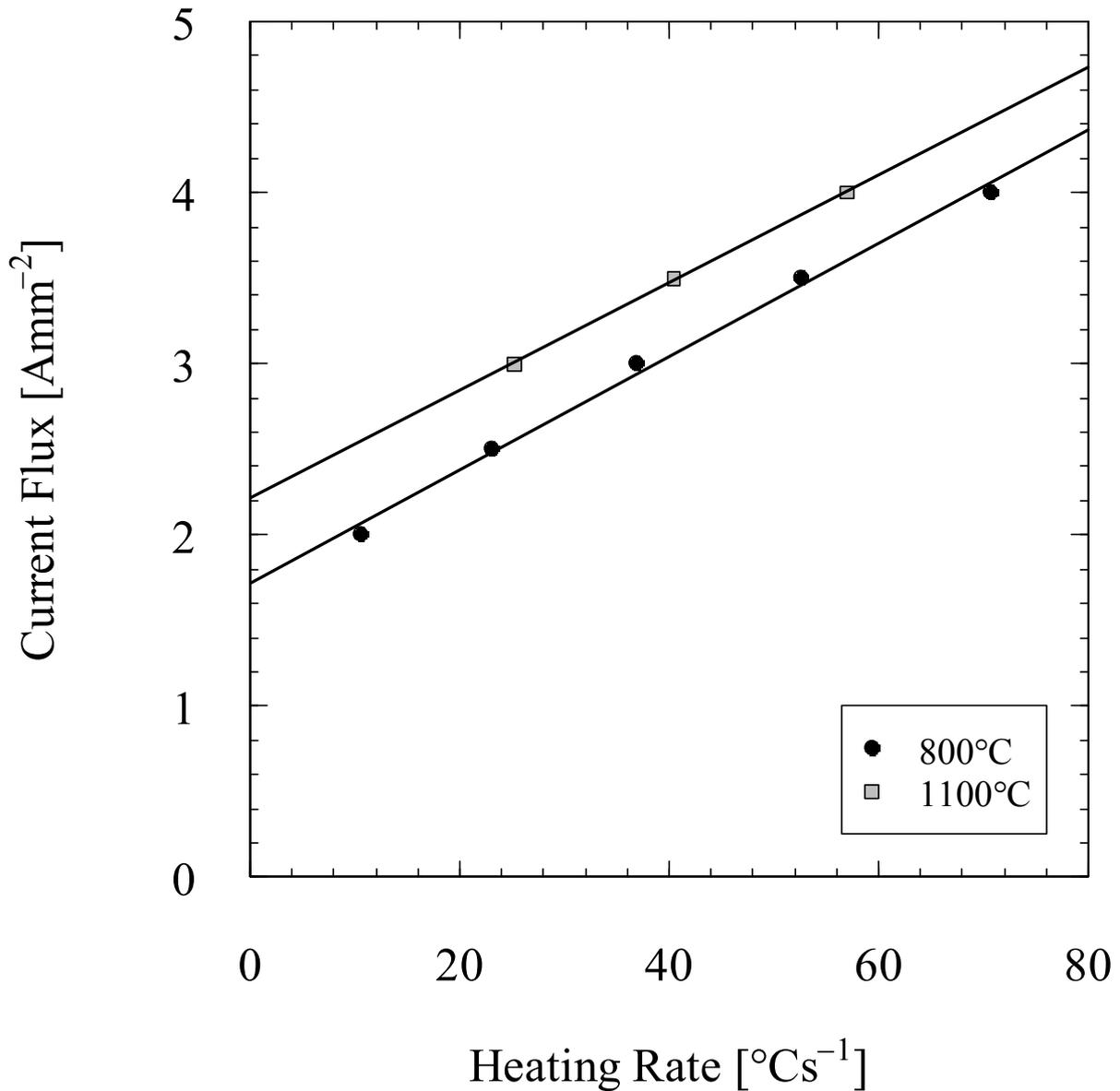
**Figure 18: Current flux required for heating rate to 800 and 1100°C from Figure 17**
