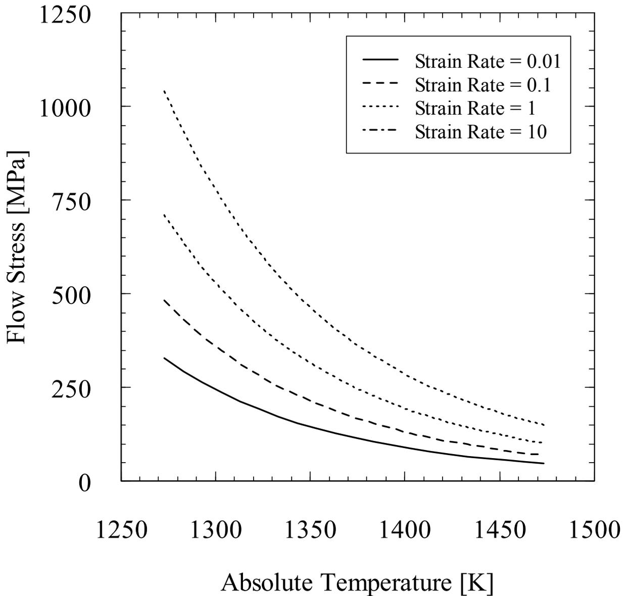
**Figure 3: Flow stress variation with temperature and strain rate for the nickel-based superalloy as defined by Equation 3**
