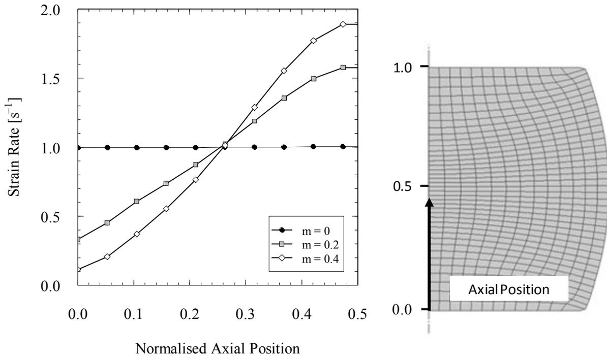
**Figure 8: Strain rate along the centreline of the isothermal model at a macroscopic true strain of 0.5 ( $T=1100^{\circ}\text{C}$ ,  $\dot{\epsilon}=1\text{s}^{-1}$ ,  $\epsilon=0.5$ )**
