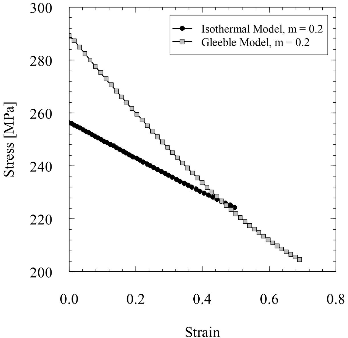
**Figure 27: Comparison of stress-strain curves generated from isothermal and Gleeble models**
