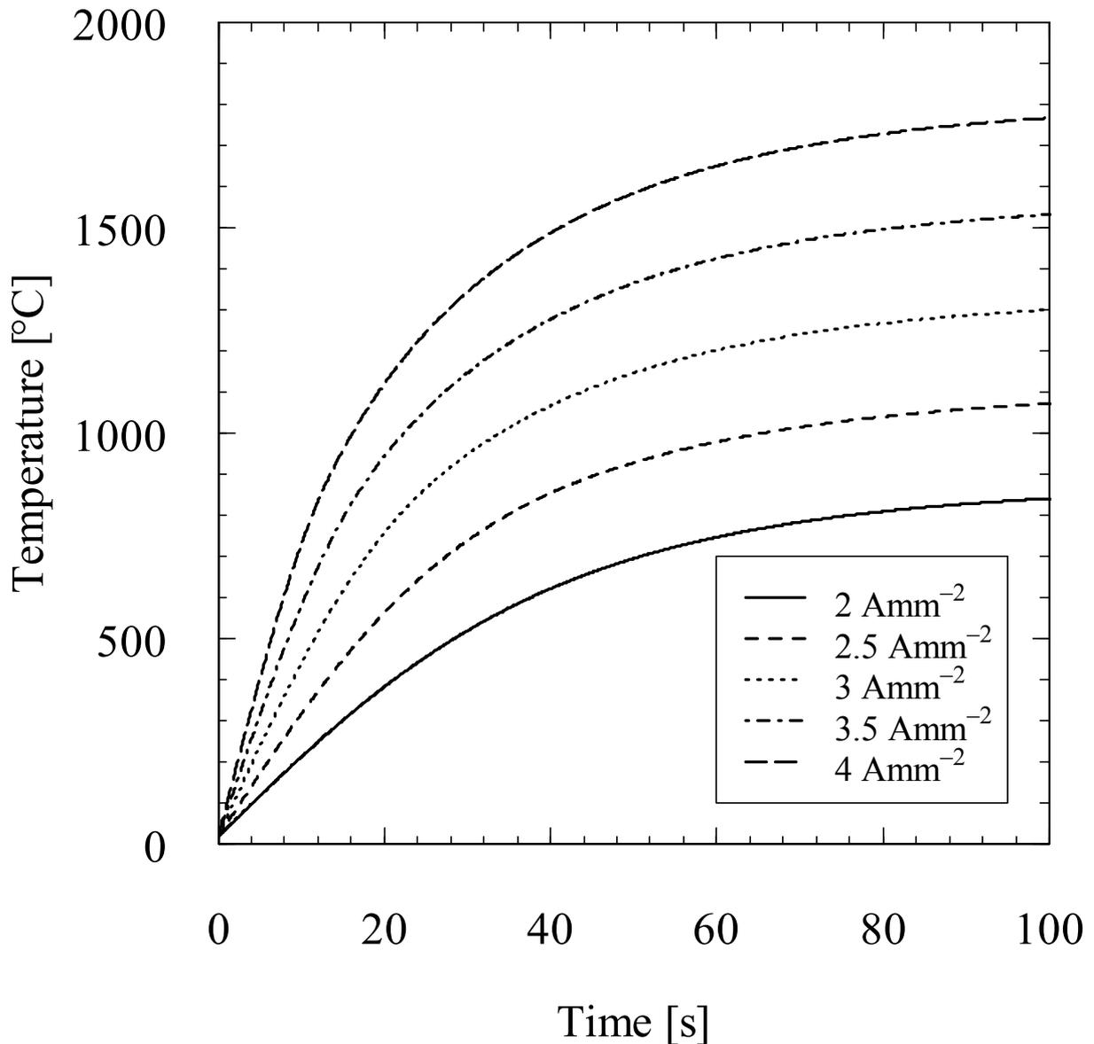
**Figure 17: Gleeble model mid-axial point temperature profiles for different applied current fluxes**
