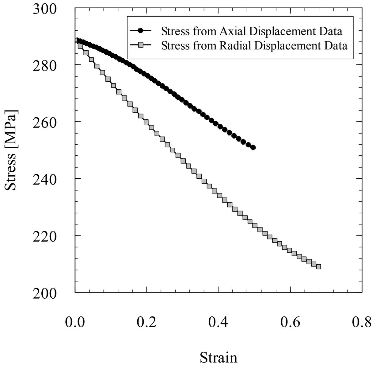
**Figure 25: Comparison of stress-strain curves derived from axial and radial displacement measurements ( $T=1100^{\circ}\text{C}$ ,  $\dot{\epsilon}=1\text{s}^{-1}$ ,  $m=0$ ,  $\eta=0.9$ )**
