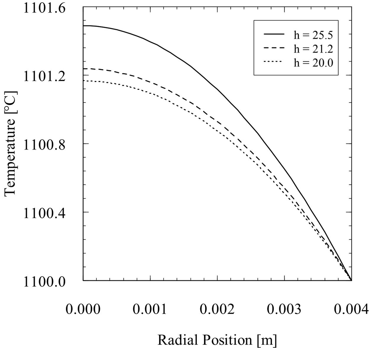
**Figure 14** Theoretically-calculated radial temperature distribution in the Gleeble specimen at 1100°C assuming steady-state conditions for different values of  $\bar{h}$
