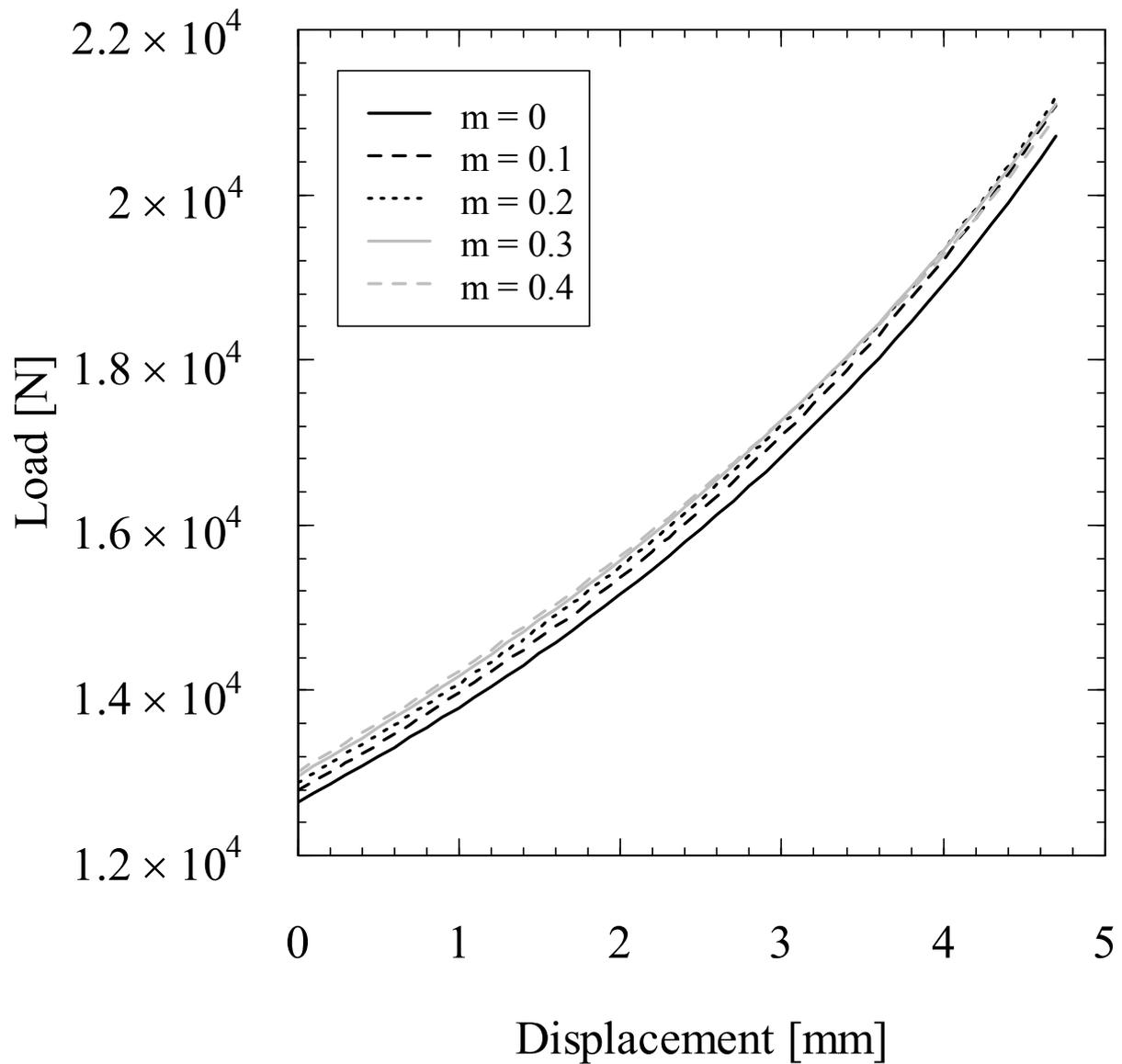
**Figure 5: Effect of  $m$  on load-displacement results from isothermal model ( $T=1100^{\circ}\text{C}$ ,  $\dot{\varepsilon}=1\text{s}^{-1}$ )**
