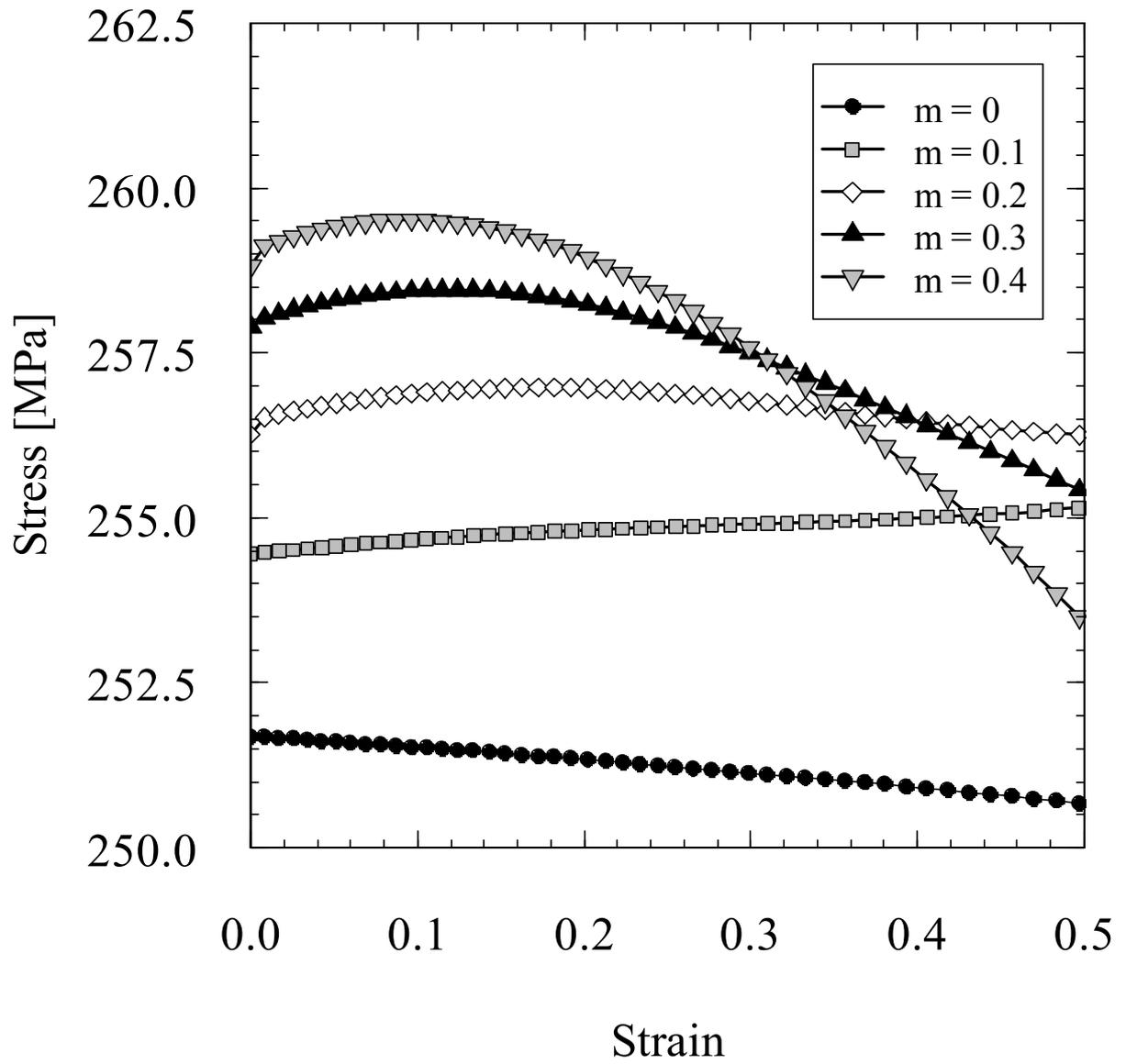
Figure 6: Effect of  $m$  on stress-strain curves from isothermal model ( $T=1100^{\circ}\text{C}$ ,  $\dot{\epsilon}=1\text{s}^{-1}$ )
