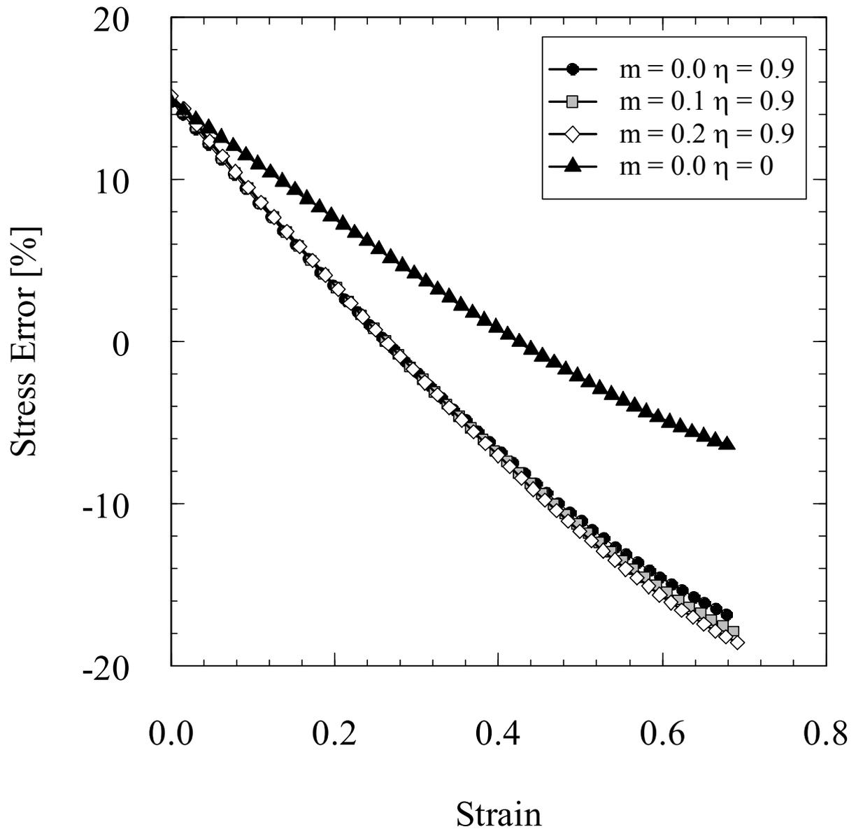
**Figure 26: Comparison of relative stress errors from Gleeble compression models ( $T=1100^{\circ}\text{C}$ ,  $\dot{\epsilon}=1\text{s}^{-1}$ )**
