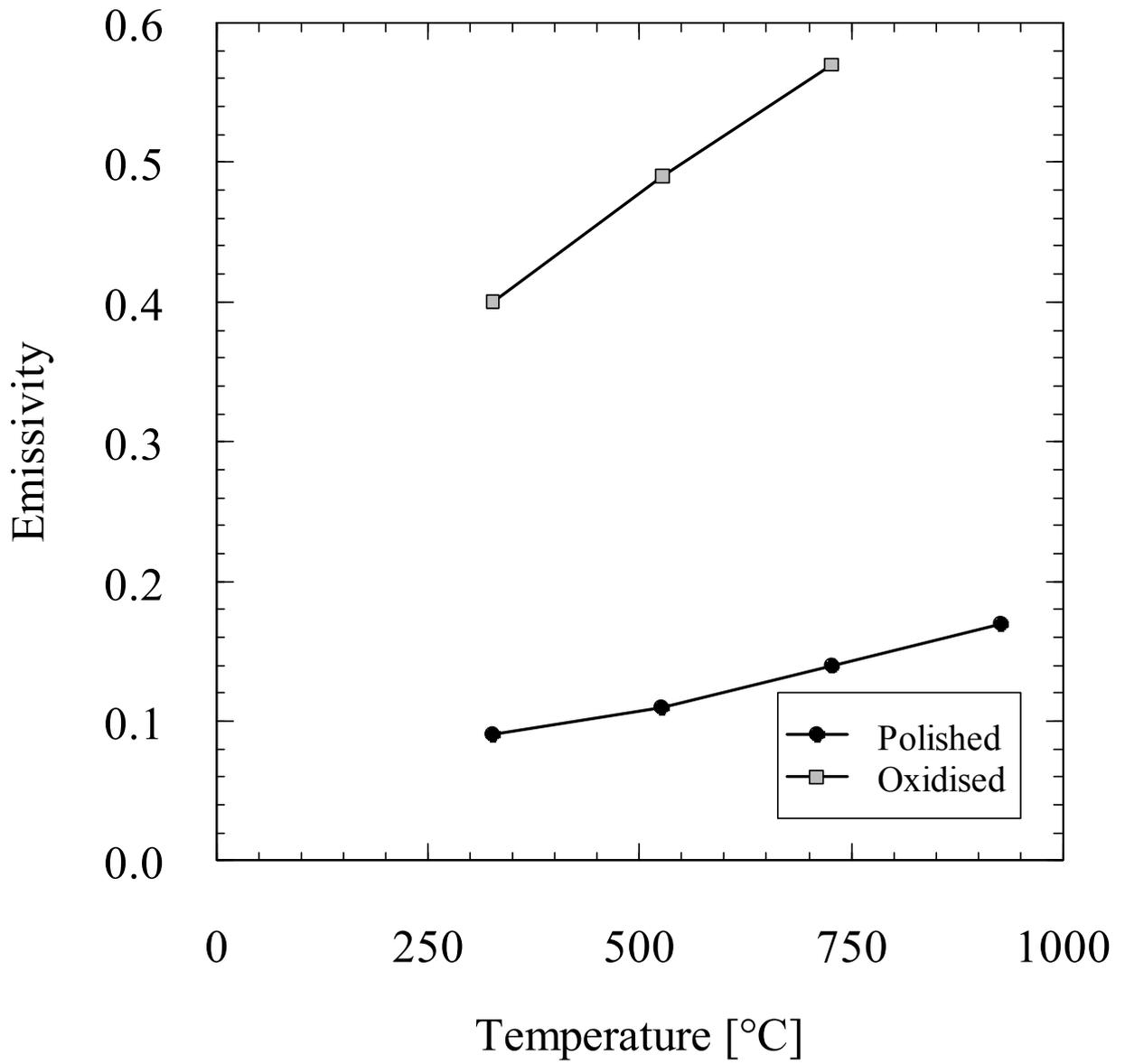
**Figure 12: Temperature dependent emissivity values for pure nickel [14]**
